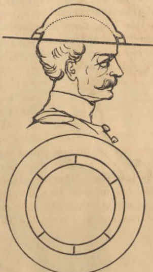
Fig. 7. Sectional views of the Ventilated Hat.
